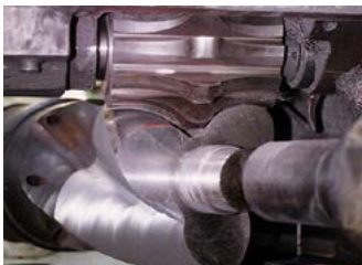
● Rotor processing using a milling machine
